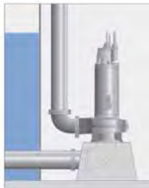
CT - A vertically-mounted, permanent dry well or in-line installation with flange connections for suction and discharge pipe work.
